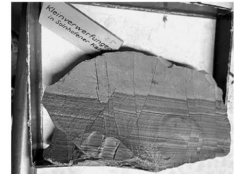
Fig. 11: Minute fractures in Sollnhofen limestone: cracks are immortalized in the rock as line drawings
