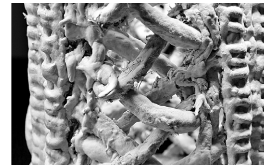
Fig. 18: Myko-Plektonik explores the filamentous fungal growth on Structural Textiles
