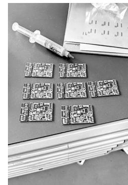
Fig. 10: Circuit board for monitoring indoor climate and gas compositions
